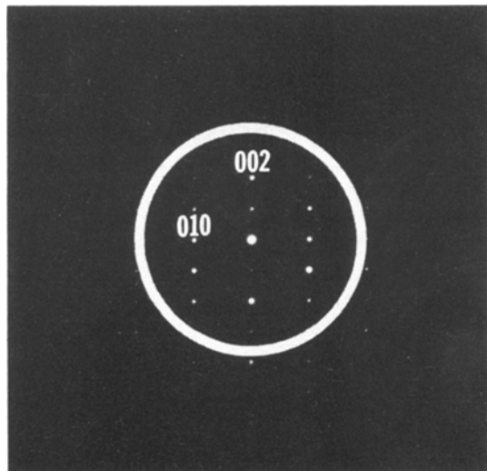
Figure 5 [10.0] electron diffraction pattern of 2H AlN; the size of the objective aperture has been indicated.
